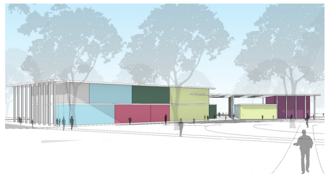
Figure 6.4: Conceptual design option uses multiple roof heights to provide rooftop terraces and hide equipment.
