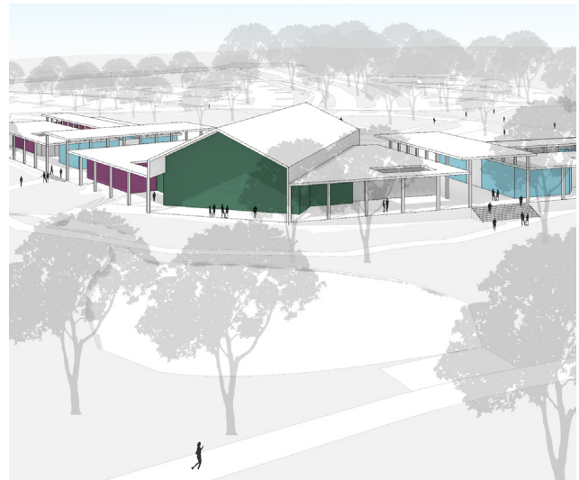
Figure 6.3: Conceptual design option uses columns along the south facade and for breezeway corridor to create a unifying facade aesthetic.
