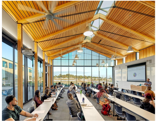
Use of transparency, exposed natural materials, and lighting/fan systems to create an inspiring and high-performing classroom space.
